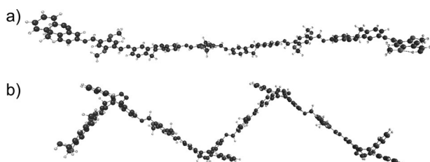
Figure 2. Optimized geometry of short polymer chain (PM3) before (a) and after (b) reaction with phenyl azide. Note the accordion-like contraction of the polymer backbone.
